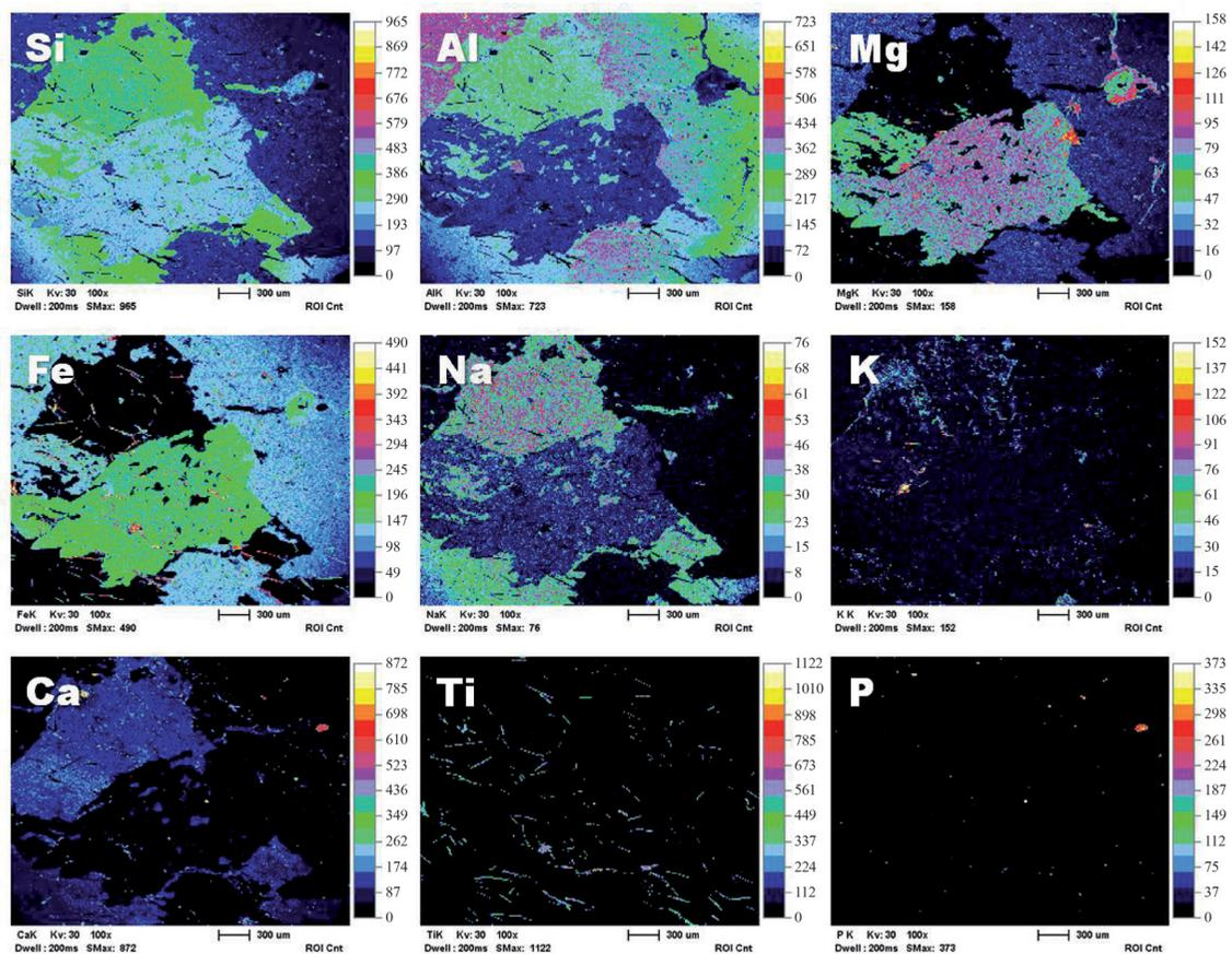
**Figure 7.** Si, Al, Mg, Fe Na, K, Ca, Ti and P compositional maps of the staurolite metabasites. Light colors show areas of high concentration while dark colors represent areas of low concentration (black is very low concentration).
