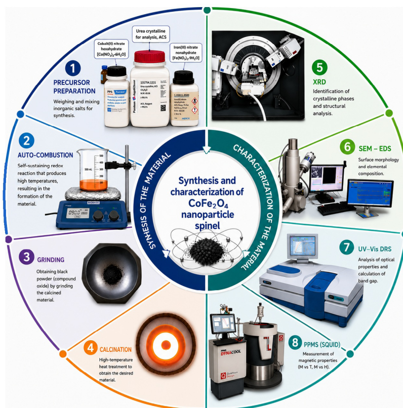
Figure 1. Graphical scheme of the synthesis process and the characterization of the CoFe 2 O 4 nanoparticles
