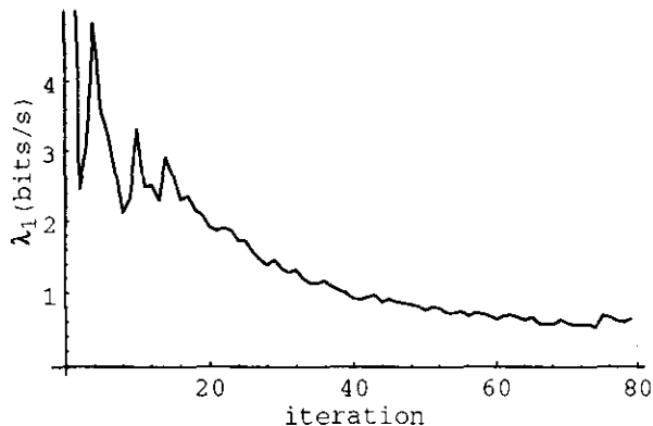
Figure 8. Typical converging result of the Wolf et al. (1985) algorithm.
