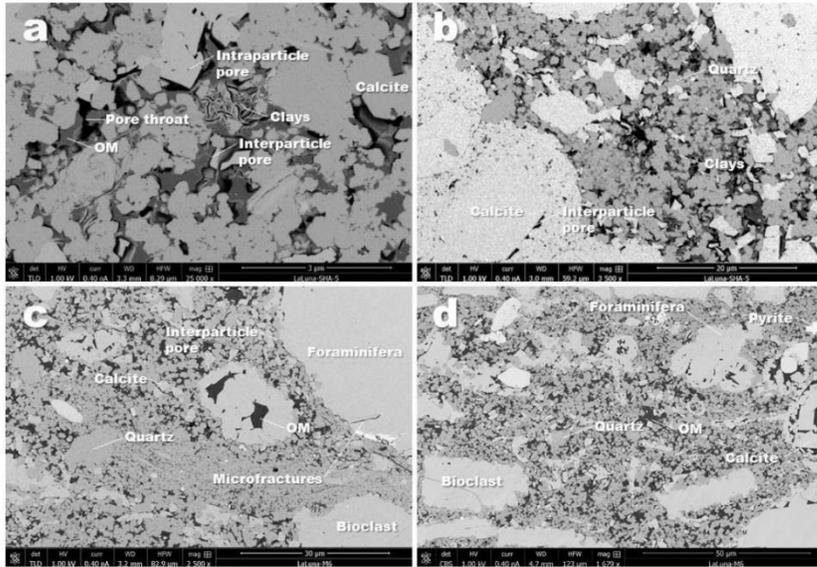
**Figure 8S.** Organoporosity in nonlaminated to slight laminated foraminifera wackestones of the Galembó Member.
