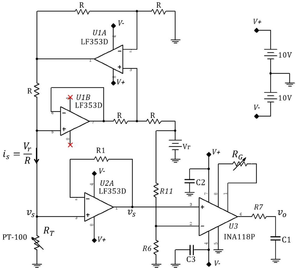
**Figure 6S.** PT-100 sensor conditioning circuit
