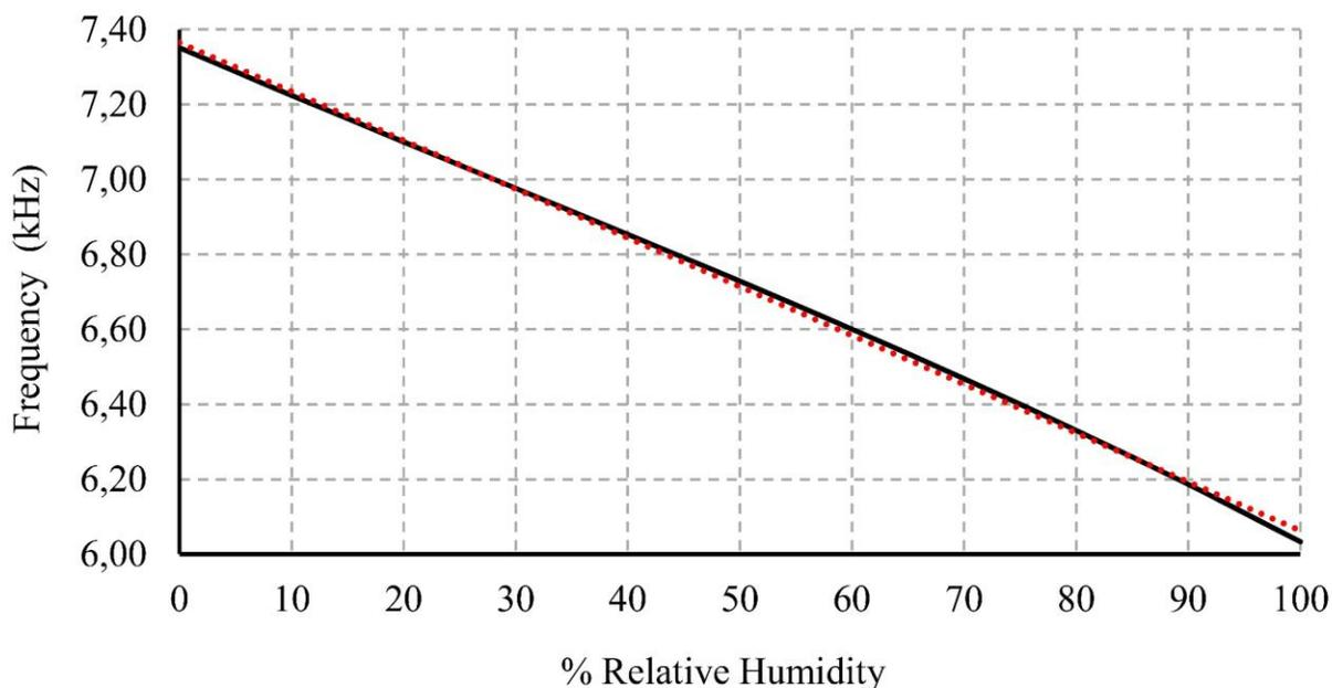
**Figure 3S.** frequency response of the *HS1101*
