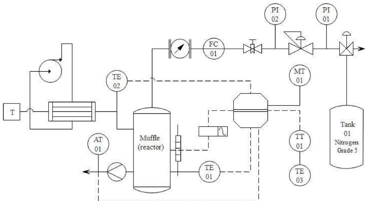
**Figure 1S.** P&D diagram pyrolysis system
