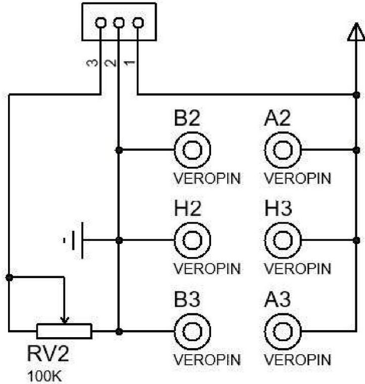
**Figure 4S.** Schematic diagram of the circuit MQ135 sensor
