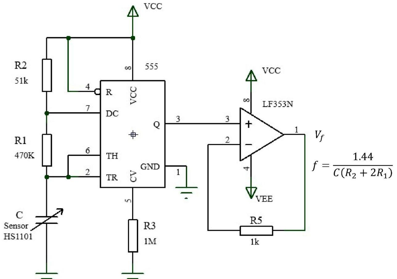
**Figure 2S.** HS1101 sensor conditioning circuit
